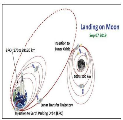
satellites, will place the mooncraft in the Earth Transfer Orbit approximately 16.2 minutes after take-off. This will be the first operational flight of GSLV-Mk-3.
