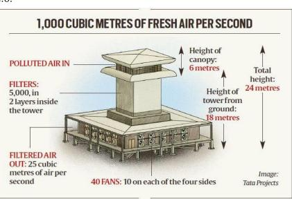
Inside the tower in two layers are 5,000 filters. The filters and fans have been imported from the United States.
